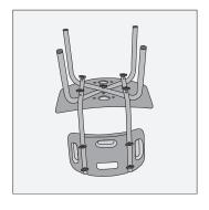
**NOTE:** Seat depth can be adjusted by chosing 1 of the 2 holes on the frame supports.
