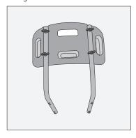
4. Attach backrest to the seat by aligning holes on "L" shaped frame supports with the holes on the leg sections. Secure in place using the longer thumb screws, making sure to pay attention to the "rear" of the seat marked on the bottom of the chair.
