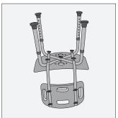
1. Before use, adjust height of each leg to your specific needs, making sure all legs are at the same height. When desired height is reached, lock legs into place by aligning buttons into proper holes, per illustration.
