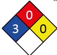
Note: The hazard category numbers found in GHS classification in section 2 of this SDSs are NOT to be used to fill in the NFPA 704 diamond. Blue = Health Red = Fire Yellow = Reactivity White = Special (Oxidizer or water reactive substances)
